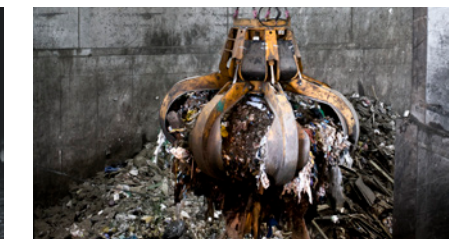
3. GRAPPLES Hardox 450 or 500. Hardox can significantly increase the life of the grapple and other gripping equipment.
