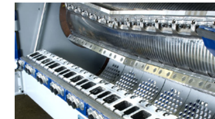
5. GRANULATOR KNIVES Hardox 600 or Extreme. Granulator knives are used for the fragmentation of waste especially plastic, tires, cables and rubber waste. The high toughness of Hardox steels provides substantially higher resistance against chipping.
