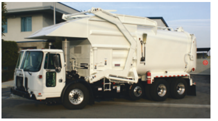
1. GARBAGE TRUCK Hardox 400 or 450. With the increased hardness of Hardox, lighter trucks with higher payloads can be produced. For packer blades inside garbage trucks, Hardox 450 or 500 is used.
