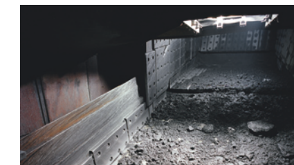
2. LINER PLATES Hardox 500, 550 or 600. Hardox can be used to line the walls of the sorting pockets.
