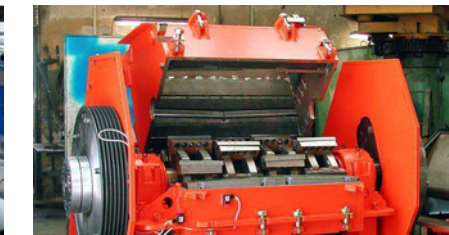
6. PRISMATIC KNIVES Hardox Extreme or 600. For the fragmentation of waste, especially plastics, tires, cables and rubber waste, Hardox can be used. The high toughness of Hardox steels provides substantially higher resistance against chipping.
