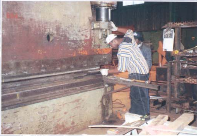
▲ 400 ton pressbrake x 14-ft. forms items such as expansion joints, transitions, chutes, tube shields, eccentric and concentric cones, and pulverizer wear parts.
