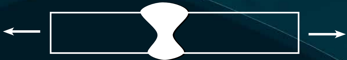
Figure 5: Different types of tensile specimens for testing of welded joints.
