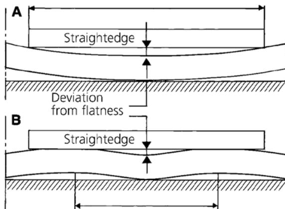
The maximum permissible vertical heights for each tolerance class, thickness and measurement length are specified in the table below. Tolerance class S is applied only subject to special agreement.
